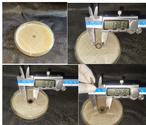
Figure 2: showing DIZ on day 7 of control, silver nanoparticles, copper nanoparticles, graphene oxide nanoparticles
