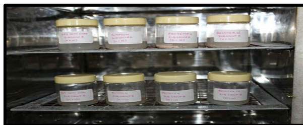
Fig 4: Total 80 Specimens in Artificial Saliva stored in Incubator at 37°C.
