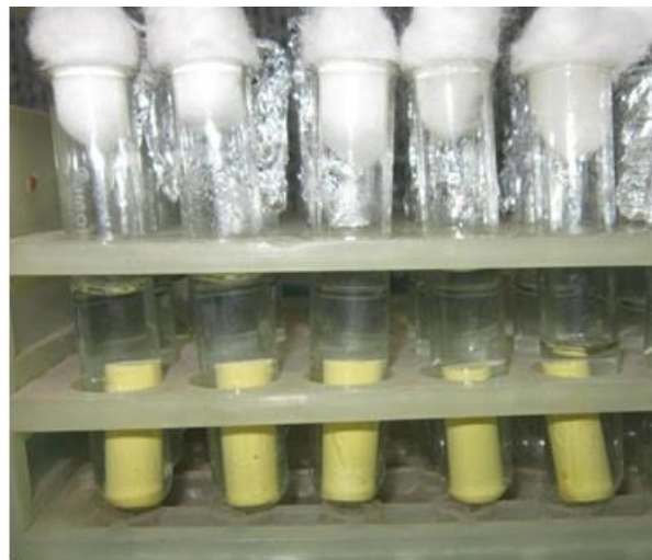
Fig 3: Dental stone cylinders dipped in sterile phosphate buffered saline.
