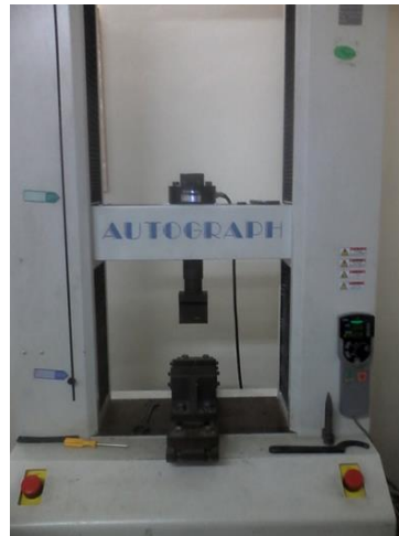
Fig 7: Universal Instron testing machine (Model no. Autograph AG 15, Shimadzu, Japan)
