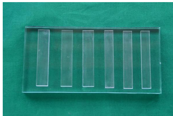
Fig 1: Acrylic specimens assembly on glass slab.
