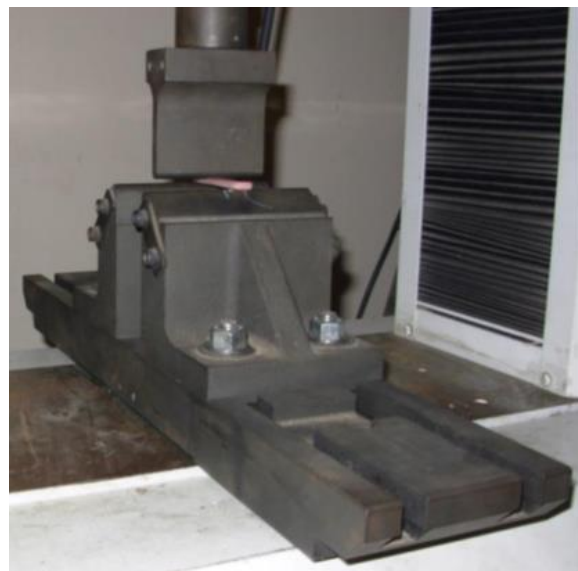
Fig 8: Sample testing of Flexural strength.
