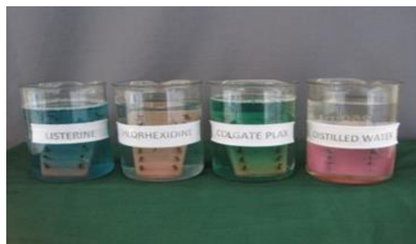
Fig 2: Two sample along with jig inserted in test solution.
