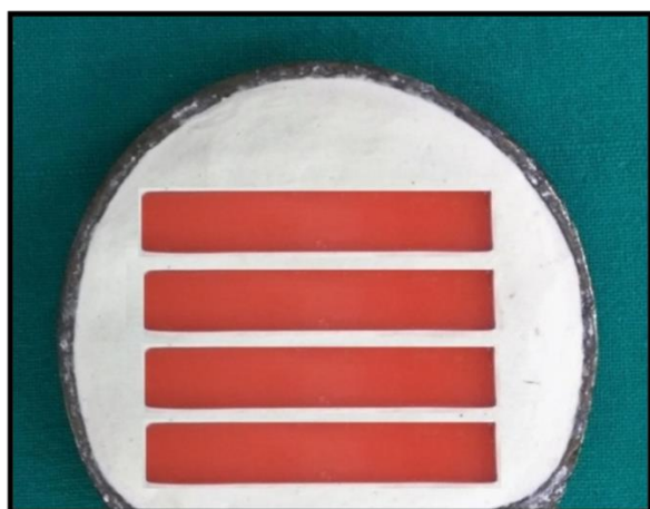
Fig 3: Wax molds flaked with plaster in the flask.
