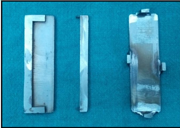
Fig 1: Stainless steel mold measuring 65mm x10mm x2.5mm.
