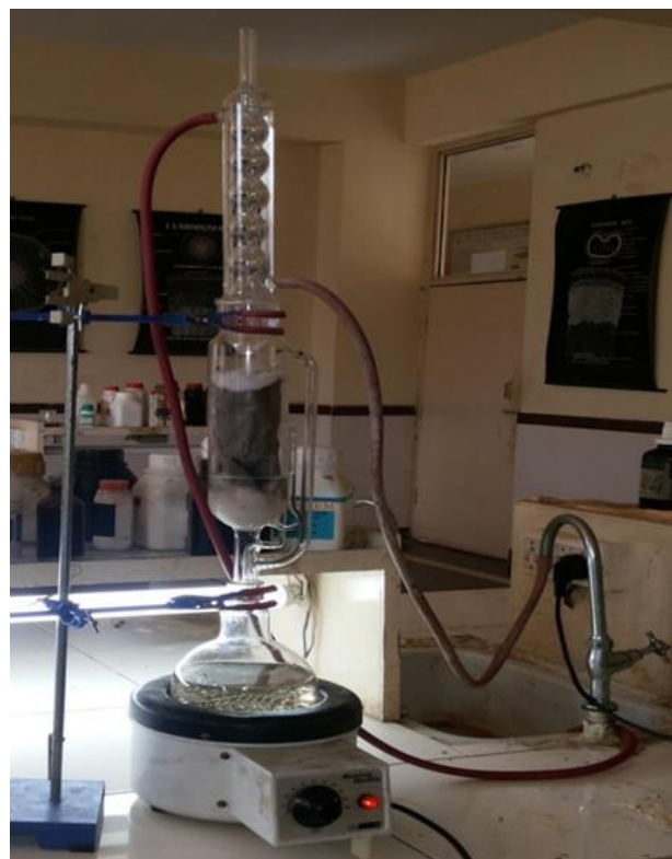
Fig 4: Soxhlet extraction process for water extract.
