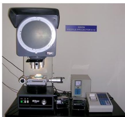
Fig 7: Cast being measured on profile projector.
