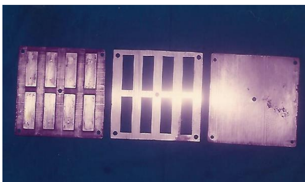
Fig 2: Photograph showing metal mould used for preparation of acrylic resin specimens with and without liners.
