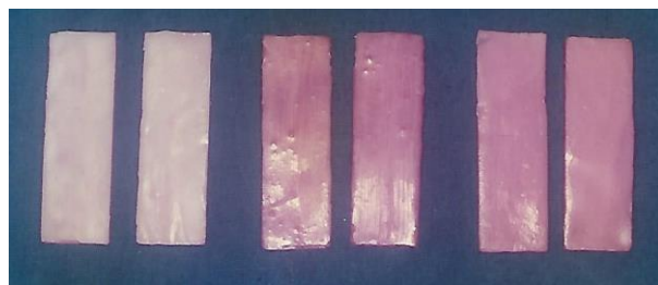
Fig 4: Acrylic resin specimen with soft liners 'Coe Comfort, Visco gel, Orthogel' respectively.
