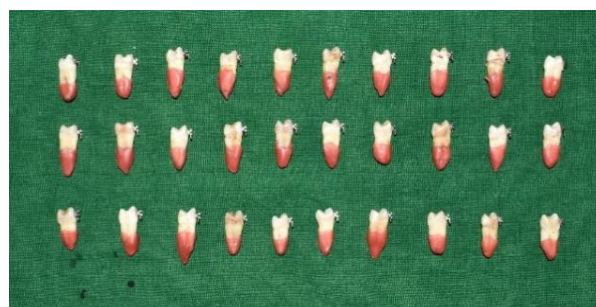
Fig 2: Samples after bonding sealed with sticky wax of group A, B & C.
