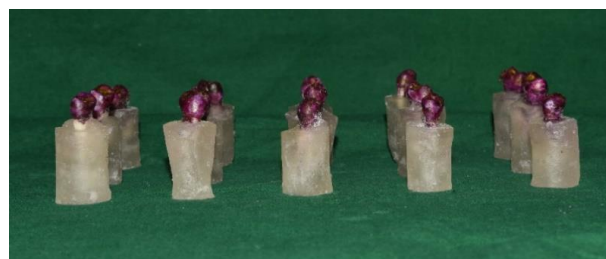
Fig 3: Samples after dying embedded in acrylic in group A, B & C.
