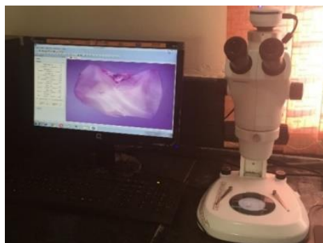
Fig 5: Digital Stereomicroscope (Model -SMZ25 Nikon - 15 X)
