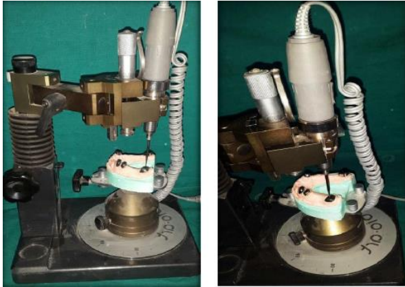
Fig 8: Primary copings were milled on a surveyor to attain parallelism between the copings. Secondary telescopic copings were fabricated over the milled primary copings.
