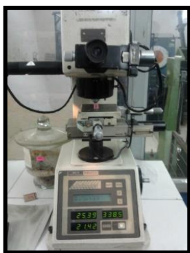
Figure 4: Testing of samples by Digital Vickers Microhardness Tester
