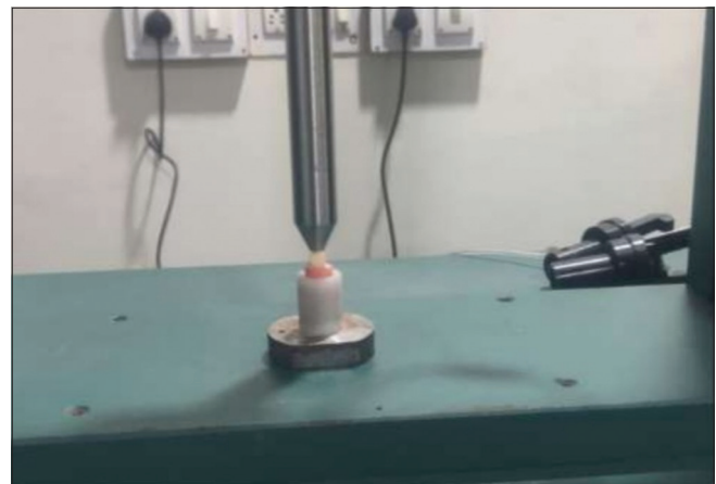
Figure 2: Testing of specimen using universal testing machine
