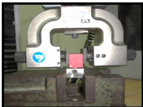
Fig 14: Tensile bond strength testing of the sample.
