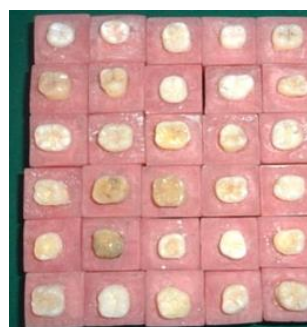
Fig 3: Mounting of teeth in auto polymerizing resin.
