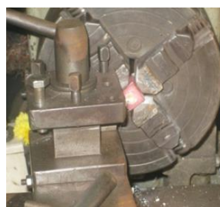
Fig 4: Preparation of natural tooth using precision milling lathe.
