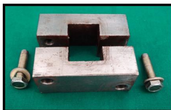
Fig 2: Stainless steel mold for mounting.
