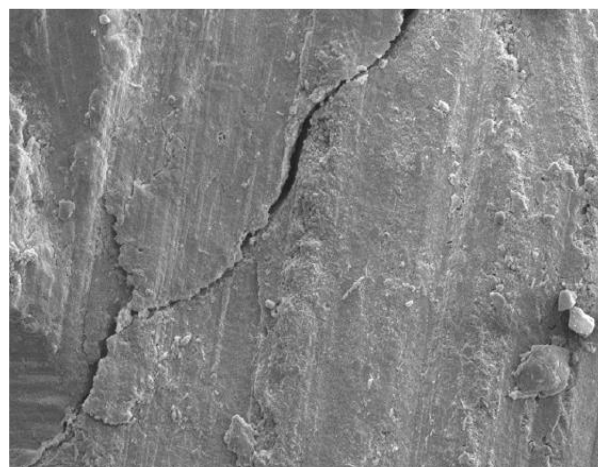
Fig 1: Field emission gun-scanning electron microscope image of gap at the dentin-furcation repair material interface of Biodentine
