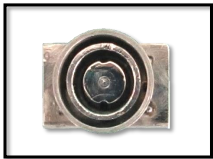
Fig. 1 (b):Master Die with Impression Sleeve and Pattern Sleeve.
