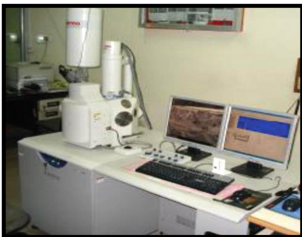
Fig 9: Scanning Electron Microscope (HITACHI Model: 3400N).
