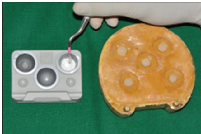
Figure 7: Application of polymer ball on bonding surface
