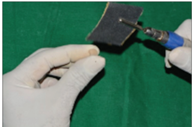
Figure 3: Group 1 surface treatment using 220 grit dry and wet sand paper on bonding surface
