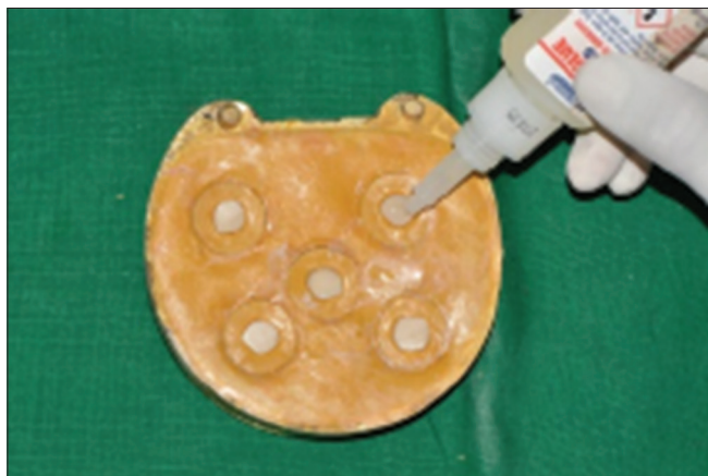
Figure 5: Group 3 cyanoacrylate application directly on bonding surface with help of dispensing bottle
