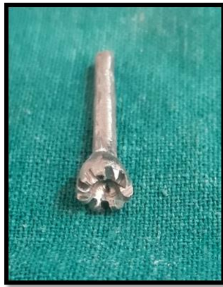
Fig 6: Specialized drill for fabrication of suction cups.
