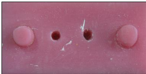
Fig 16: Relief holes created in counter block.
