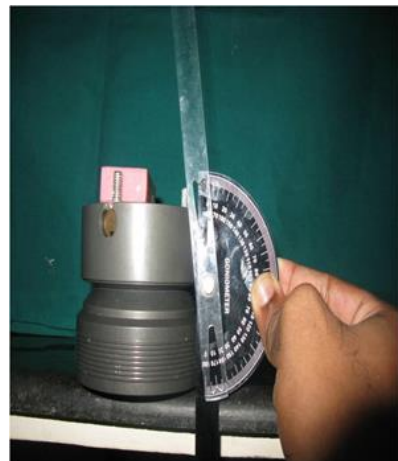
Fig 6: Acrylic block stabilized at 10 degree and angulation is verified goniometer.
