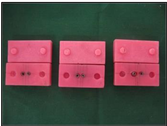
Fig 9: Implants placed and stabilised using acrylic resin.
