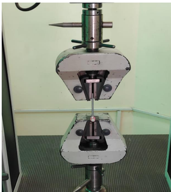
Fig 6: Shear bond strength testing in universal testing machine.
