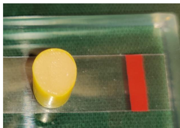
Fig 4: Dentin substitutes layered by composite resin after application of universal adhesive.
