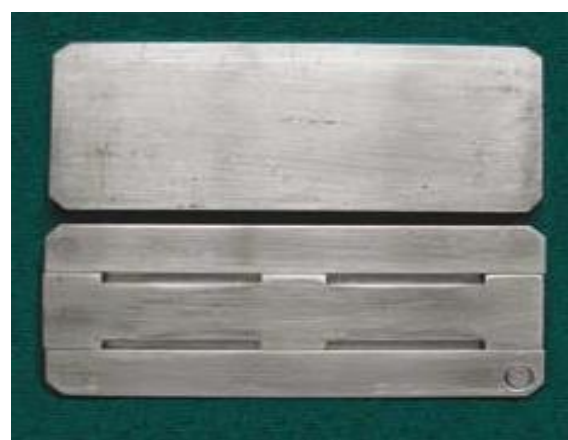
Fig 1: Aluminium split mold for making specimens.
