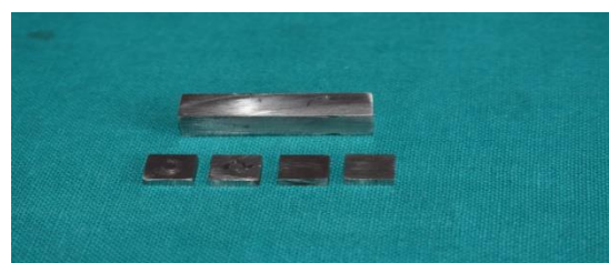
Fig 1: Stainless steel (S.S.) steel master die (10*10*40MM).
