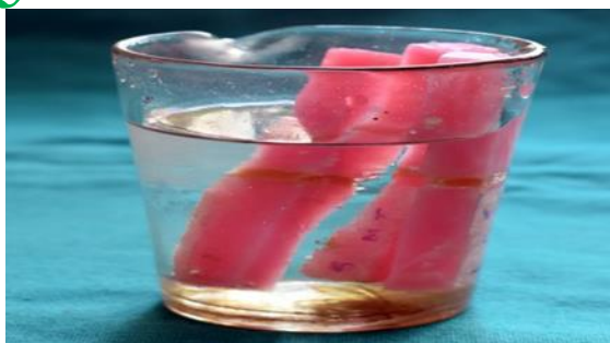
Fig 5: Test specimen immersed in artificial saliva for 7 days.
