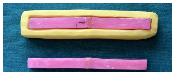
Fig 3: fabrication of UFI GEL P specimen.
