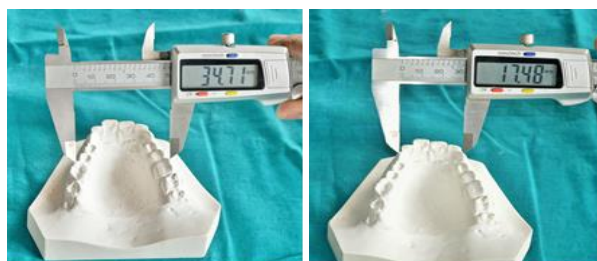
Fig 3: Measurements taken using 150mm Digital Caliper (Workzone)
