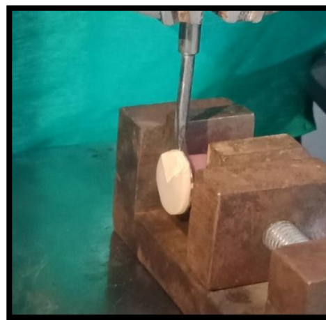
Fig 9: Load application for shear bond testing
