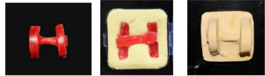
Figure 4. Wax buildup, impression of the finalized wax contour and gypsum replica used to fabricate the hollow component.
