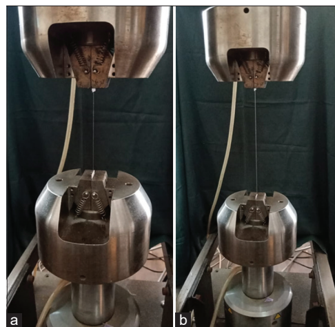
Figure 3: Suture material in (a) non-tensioned state and (b) while tensile loading
