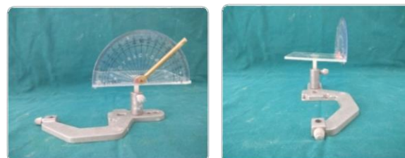
Fig 3: The device to measure the angle formed with horizontal plane.
