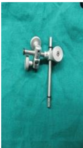
Fig 3: Transfer clamp assembly with transfer rod, transverse clamp and No. 1,2,3 thumbscrews.
