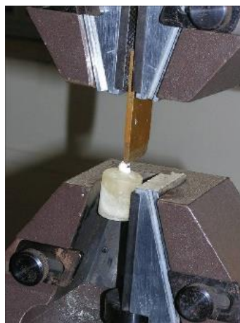
Fig 4: In the upper jaw of the instron machine a metal plate with sharp edge was attached which transferred the force onto the bracket as shown.
