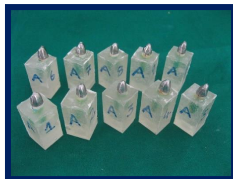
Fig 7: samples embedded in acrylic blocks.
