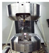
Fig 4: Microshear Bond Strength Testing Assembly
