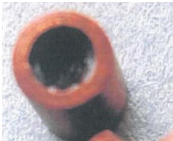
Fig 5: Copper ring used for holding core material (2mm diameter x 4mm height).
