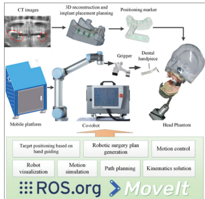
Figure 3: The scheme of the experimental HRCDIS
