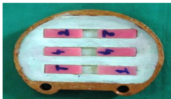
Fig 3: Repositioning of cut specimens in dental stone moulds.
