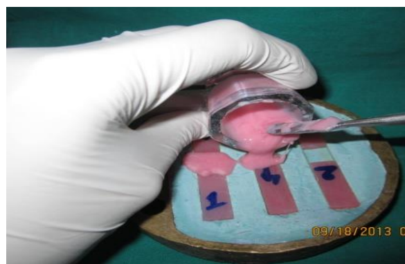
Fig 4: Addition of free-flowing repair material
