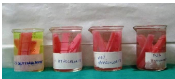
Fig 5: Disinfection of repaired specimens. [C] Flexural strength test:
