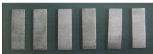
Fig 1: Master Dies of 65mm * 10mm *3mm dimension
