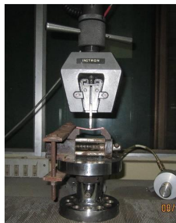
Fig 6: Transverse strength test in universal testing machine
