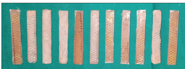
Figure 6: Bar specimens made with Triplex reinforced with metal mesh
