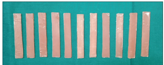
Figure 7: Bar specimens made with Triplex
