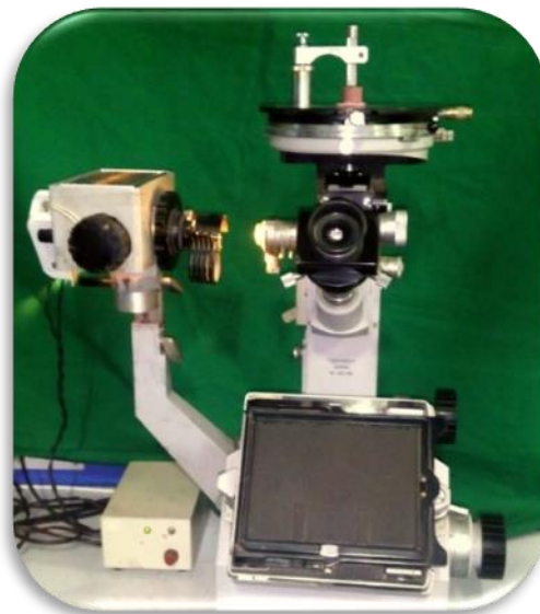
Fig 3: Samples subjected to Vickers microhardness tester (Reichert Austria Make, Sr.No.363798) for testing.
